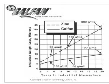
GALFAN's coated wire shows superior corrosion protection as compared with conventional galvanized coated wire. The figure on the left depicts the loss of zinc and Galfan in industrial atmospheres as measure of the relative corrosion resistance. The figure shows that the relative advantage of Galfan improves from 1.7 at five years exposure to 3.0 at the end of twenty years.
